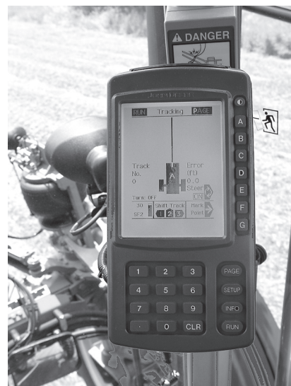
FIGURE 15. FARMERS CAN USE AUTO-GUIDANCE SYSTEMS TO APPLY FERTILIZERS ACCURATELY. SUCH SYSTEMS TIE TOGETHER GPS, GIS, AND ROBOTICS TECHNOLOGIES.
