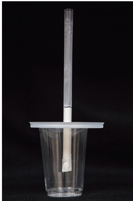
FIGURE 2.2: PHOTOGRAPH OF A COLUMN SETUP USING BABY POWDER AS A SUBSTITUTE FOR SILT. THIS COLUMN IS READY FOR WATER TO BE ADDED.
