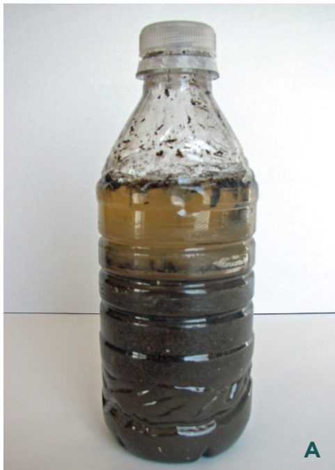
FIGURE 2.1. A. SOIL SEPARATION AFTER SITTING FOR ONE DAY
